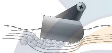
Cavitation that will cause erratic sonar readings
